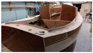
**Steves boat** progressing with internal fit out and coamings in place
