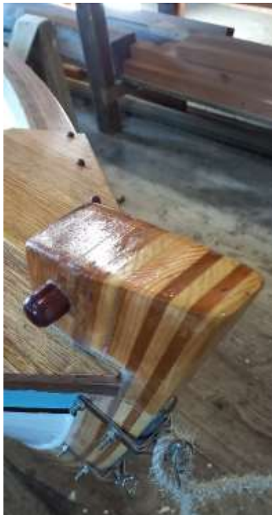
The Stem and oars show some extra detail with smart finish . Oars laminated with one Hard lamination
