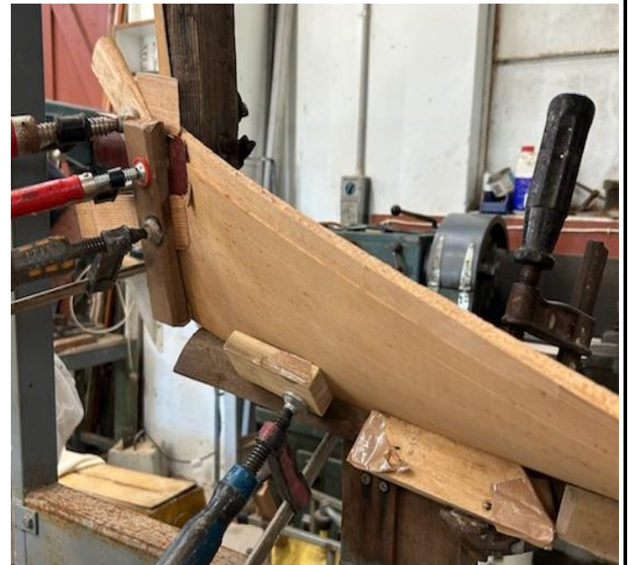
garboard plank after steaming
