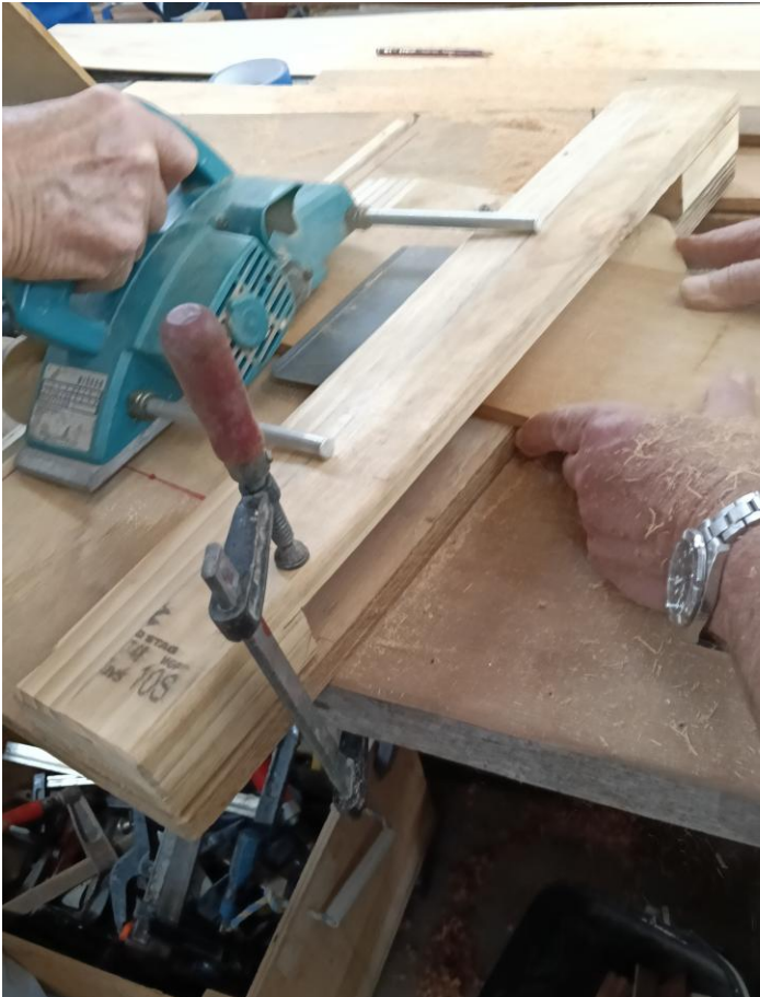
garboard plank after steaming
