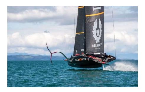
Aerospace technology — including advanced aerodynamics, lightweight materials, wind tunnel testing and advanced simulation technology — has revolutionized the sport of America's Cup racing. Today's cup-class yachts use a wing that is more akin to an airplane's wing or airfoil than to a traditional sail.
