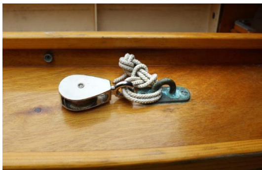
A short soft shackle connects my canoe's spinnaker sheet lead to its deck-mounted pad-eye.
